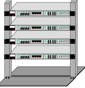
Fig 3.8 Multiple Magnum OS5116 units rack-mounted in a 23" frame
